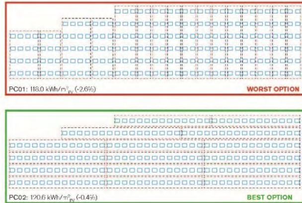
Figur 5: Southeast facade, annual estimated energy production for different panel combinations. Total PV area 308.5 m 2 , PV efficiency factor 0.15. Simulations consider the position of the sun every 5 minutes for a whole year and use typical climate data for Arlanda (Stockholm).
