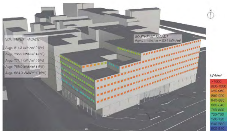
Figure 3: annual solar irradiation on the PV panels.
