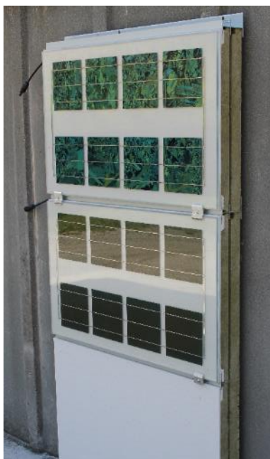
Figure 5.20: Demo-site 4, ePIZ prototypes with glass-glass PV laminate mounted on wall
