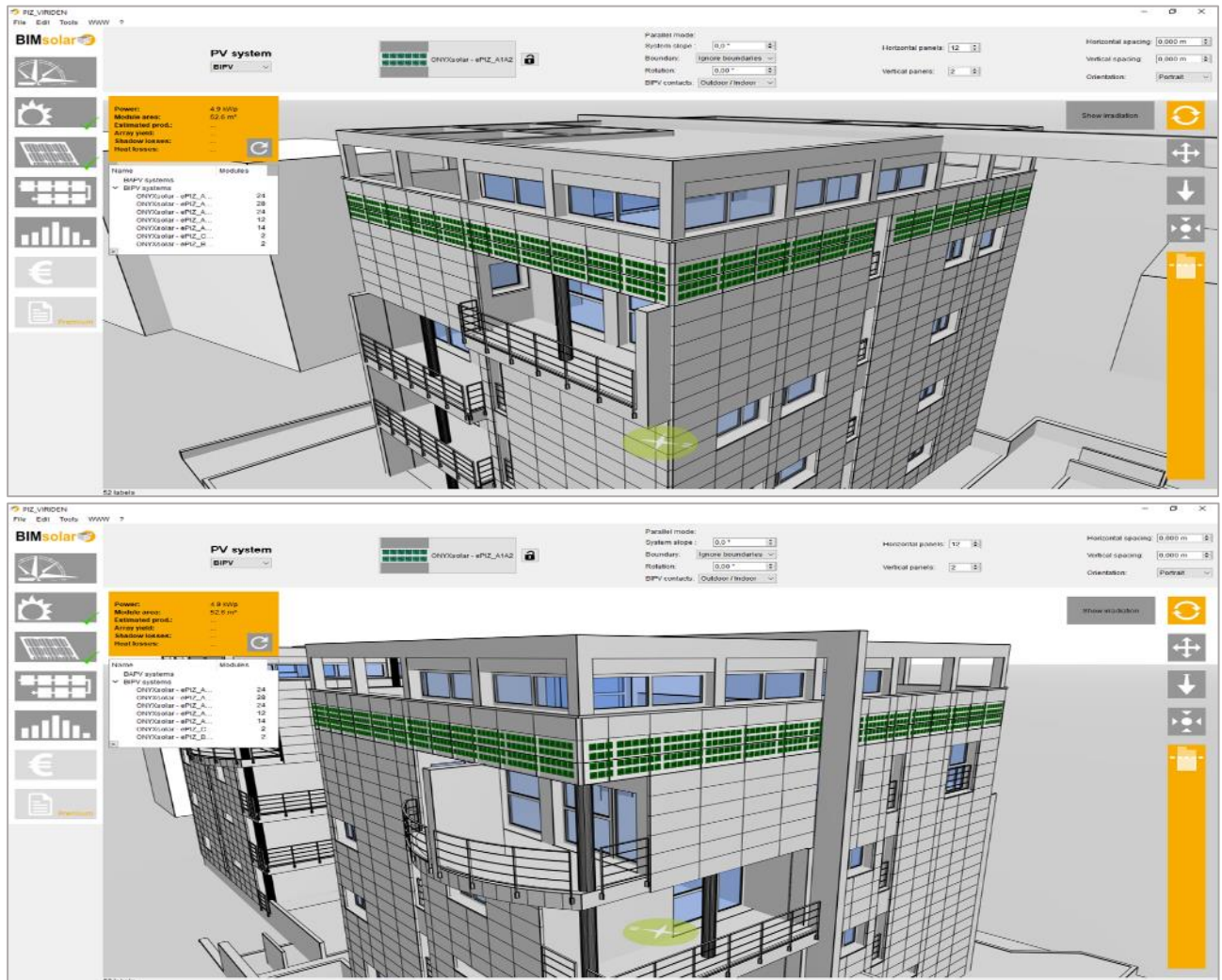
Figure 5.48: Building A – 2 rows of 1110x451mm (=102 modules) on South, East, West and North facades + 2 rows 668x451mm (=2 modules) on South-West + 2 rows of 1064x451mm (=2 modules) on North-East facades – Total 4.9kWp / 52.6sqm
