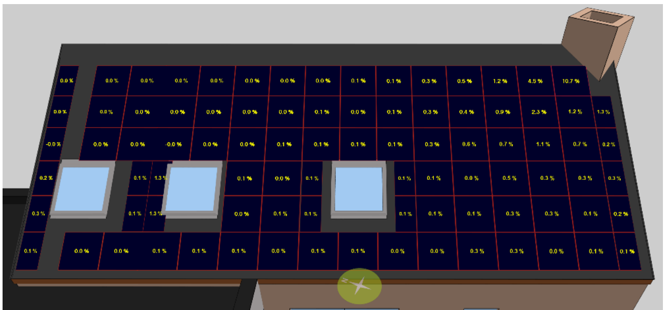
Figure 4.50: West roof – Shading losses at module level
