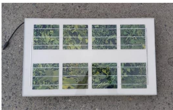
Figure 5.16: Demo-site 4, ePIZ prototype with glass-glass PV module (color of the cells is different from the one that will be installed)
