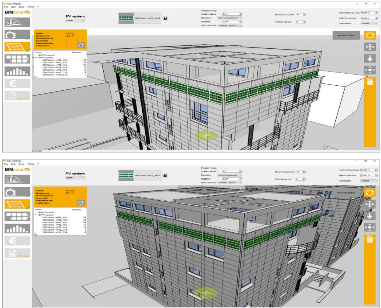
Figure 5.51: Building B – 2 rows of 1110x451mm (=102 modules) on South, East, West and North facades + 2 rows of 668x451mm (=2 modules) on South-West + 2 rows of 1064x451mm (=2 modules) on North East facades – Total 4.9kWp / 52.6sqm
