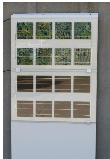
Figure 5.20: Demo-site 4, ePIZ prototypes with glass-glass PV laminate mounted on wall
