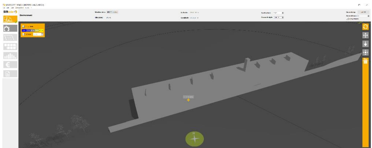
Figure 2.44 Albedo effects (reflected irradiance) are generated selecting groups and types of surfaces 50% as a setup for surroundings and for the building envelop as a general approach
