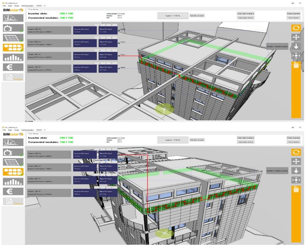
Figure 5.54: Building A - 1 inverter on each façade for all the panels (=4 inverters Azzuro-1100-TL), there is 102 module types A1&A2, 2 module types B1&B2 and then 2 C1&C2
