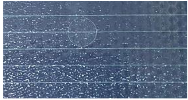
Figure 88. Detail of the circle formed on the polymer after the impact
