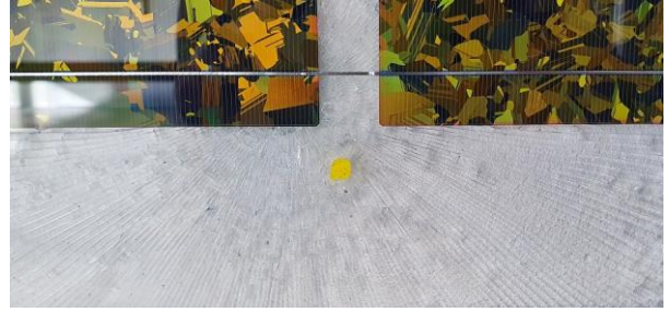
Figure 65. Hard body impact breakage of the rear glass (ID 1, position 05).
