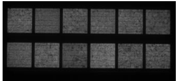
Figure 62. Electroluminescence after a hard body impact. No damages on cells.
