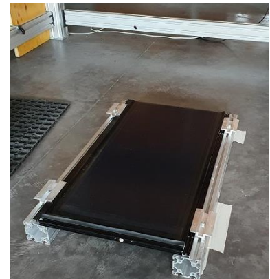
Figure 72. Temporary structure consisting of two railings on which four clamps are fixed to ensure the attachment of the module
