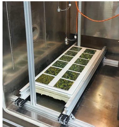
Figure 71. Structure consisting of two rails that are fixed in between the insulation layer and the mortar of the module
