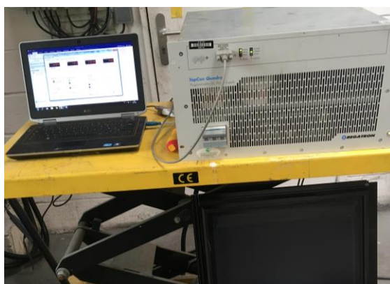
Figure 17. DC PV GENERATOR (10 kW DC) – preliminary settings before mockup connection Load device and remote control to test load on CIGS module (left) / User interface with load level (right)
