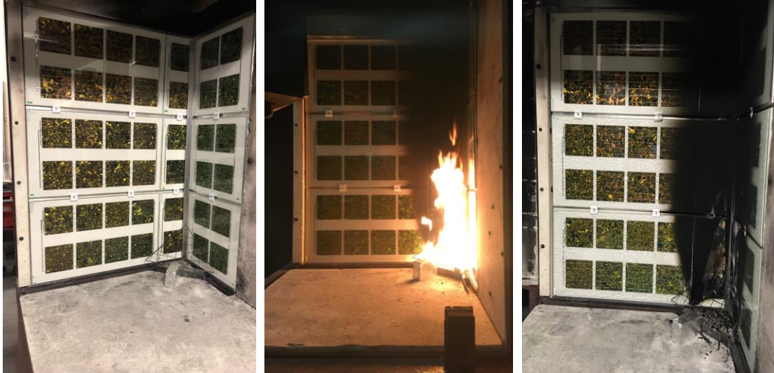
Figure 27. Before/during/after the fire test with DC PV GENERATOR load applied on veture kit cladding system with a front glass-glass module
