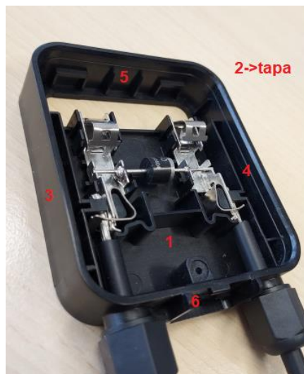
Figure 47. Picture of the reference junction box and the surfaces for view factors calculation
