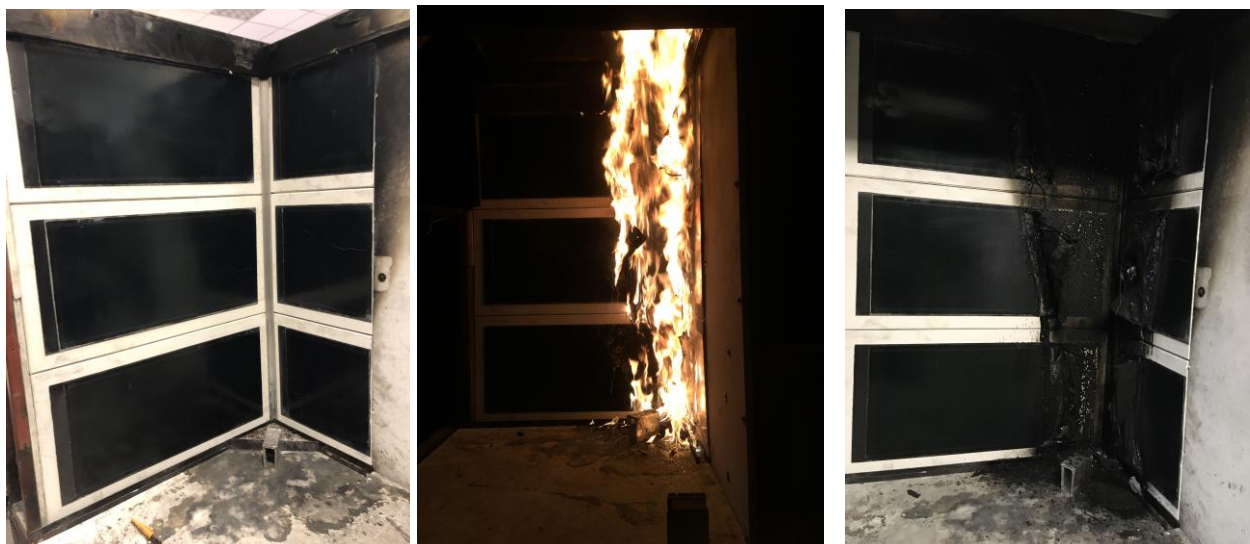
Figure 28. Before/during/after the fire test with DC PV GENERATOR load applied on veture kit cladding system with a front CIGS-based flexible module
