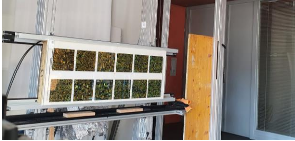
Figure 64. Hard body impact equipment.
