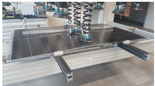
Figure 96. Test made with pull load on PV laminated glass during the cycles.
