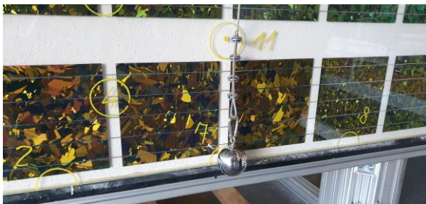
Figure 66. Hard body impact test on the edge (ID 2, position 02).
