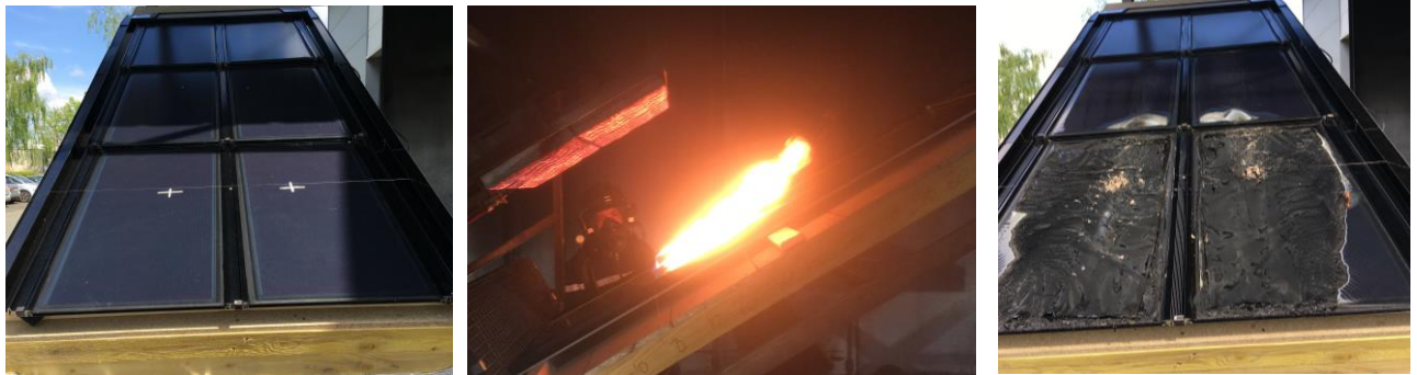
Figure 18. Before/during/after the fire test with DC PV GENERATOR load applied. During the test, current and voltage values are checked to identify possible breaks in the electrical circuit.
