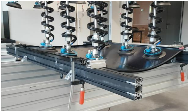
Figure 93. Deformation on PV roof tile under mechanical load.
