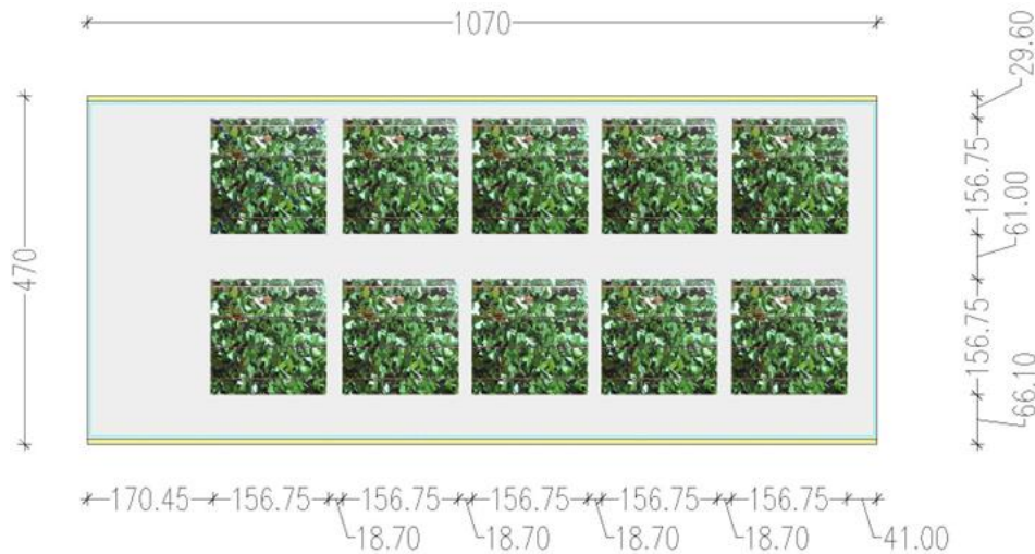
Figure 2.36: BIPV Glass-glass colored poly-Si cells module. Type B2
