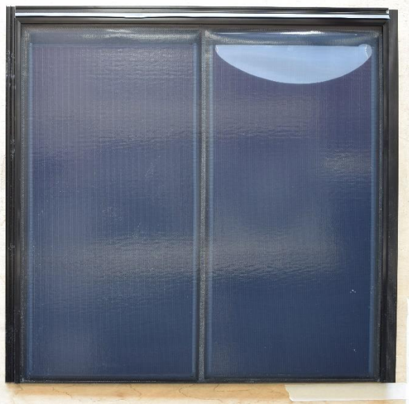
Figure 2.25: Delamination in the “new” material stack due to adhesion and thermal expansion problems in the multi-layer stack
