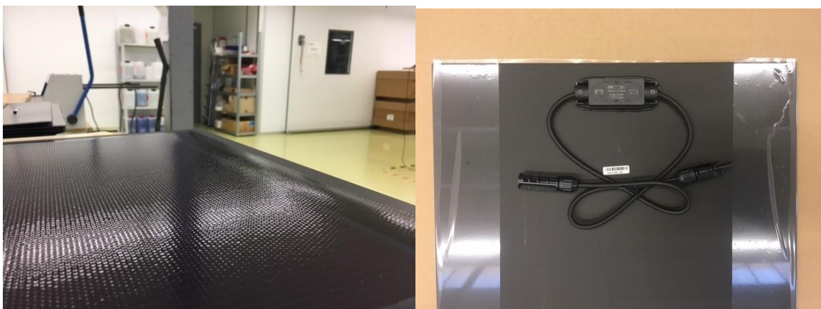
Figure 2.26: Final appearance of the module with JB on the back, protective foil and front texture imprint for anti-gloss
